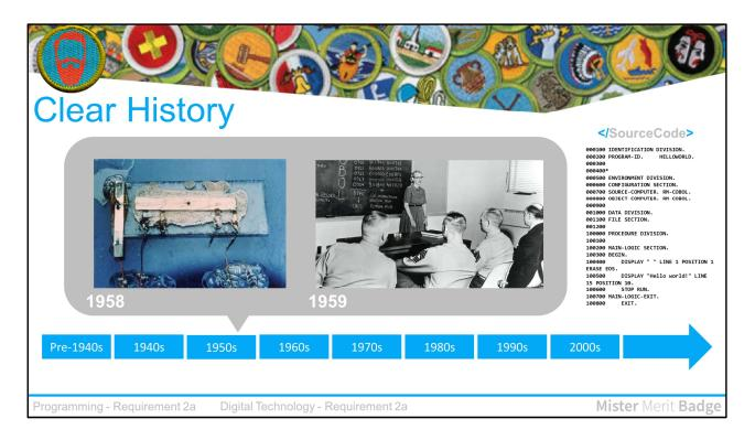
– The Integrated Circuit is invented. The integrated circuit is a set of electronic circuits on one small flat piece (or "chip") of semiconductor material, normally silicon. The integration of large numbers of tiny transistors into a small chip results in circuits that were significantly smaller, cheaper, and faster than those constructed of individual electronic components.
