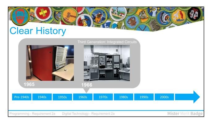
– IBM released the System/360 series of computer. The System/360 family of computers could all run the same software, but with different performances, and at different prices. The computers could be upgraded as the users' needs grew, meaning they could move up to larger computers, and still keep all of their investment in programs, data and storage media.
